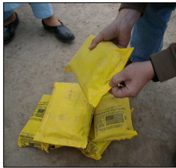
All HDR packaging had multiple splits ranging from ¼ - inch to over 2- inches in size.
